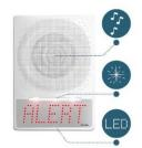
The internal wall-mounted Trio sounders are multifunctional incorporating a flashing light and an LED message display as well as the sounder. During normal schooldays the LED display shows accurate time in a digital format that is synchronised by the master clock. When an alert is activated, the display changes to a scrolling text message of up to 50 characters to visibly reinforce the audible announcement. At the same time that the alert is
